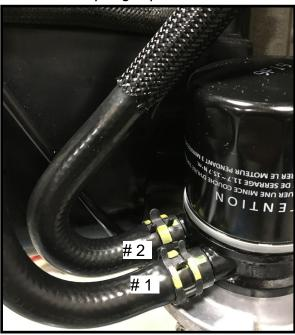
2.5 Install oil cooler hose 1 and 2 onto the oil cooler assembly using spring clips. NOTE: Position the new spring clips as shown.
