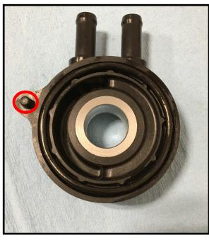
2.2 Install the adapter union bolt and filter adapter onto the crankcase cover 2 mating surface, then tighten the adapter union bolt to specification.
