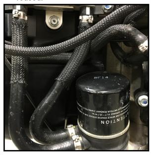
1.2 Remove the two bolts shown that secure the oil cooler assembly. The bolts will be reused.
