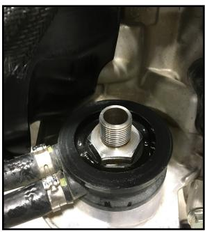
1.4 Clean the crankcase cover 2 mating surface. NOTE: The oil filter adapter locating pin aligns with the crankcase cover 2 alignment hole shown.
