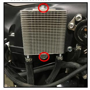
1.3 Remove the oil filter adapter union bolt and the oil cooler adapter. The union bolt will be reused.
